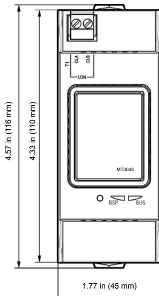
Figure 2: LONWORKS Communication Module Side View
